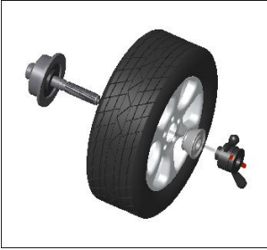
Main shaft-wheel— suitable cone( small head towards inside)—quick handle nut
