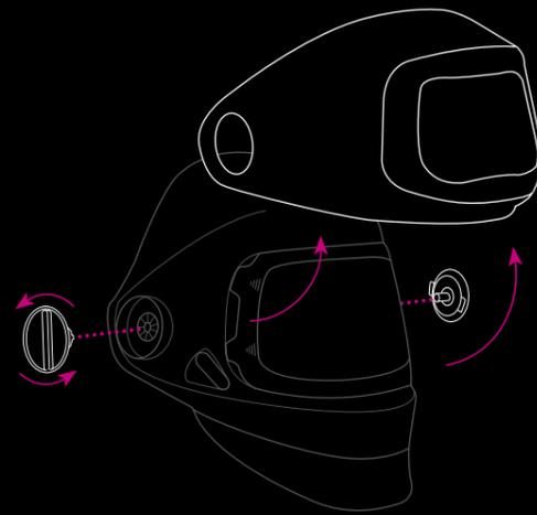
For extended non-welding work, just unscrew the two dials to completely remove the welding visor and re-attach the dials again, reducing the helmet weight by up to 36%.
