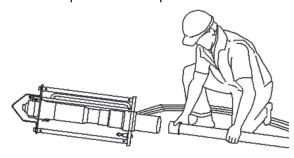
5. Lift the post and post driver to a vertical position. For long and heavy posts, two persons may be required.
