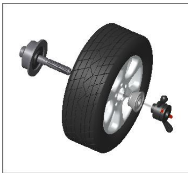
Main shaft—wheel— suitable cone( small head towards inside)—quick handle nut
