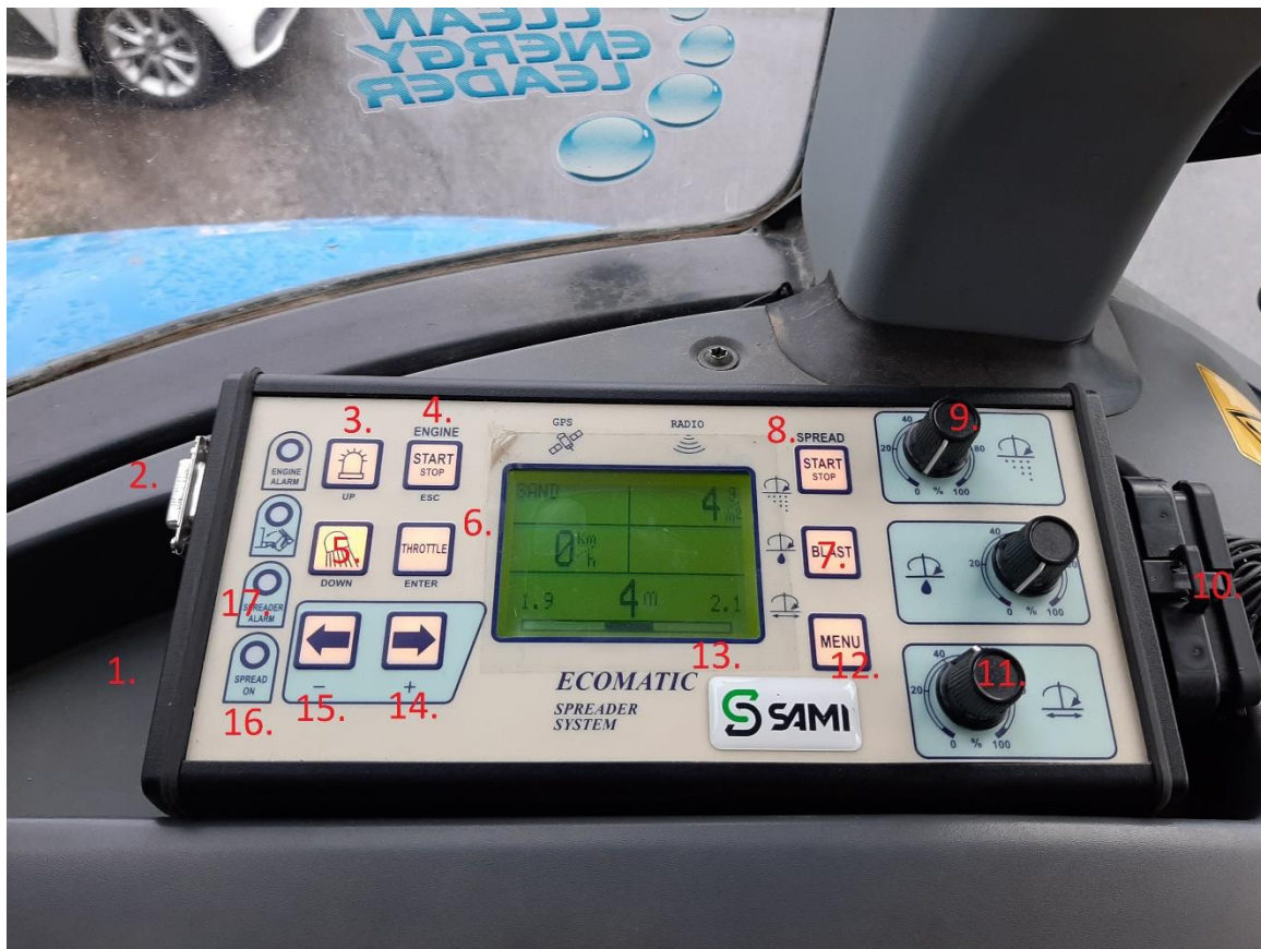
Figure 1. Control panel of the spinner spreader. (SIIA TULEB UUS PILT KORRALIKE BALLOONIDEGA)
