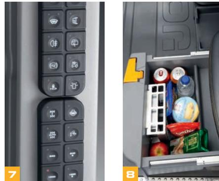
**7** Switches used less often are arranged logically on the right-hand cab pillar – out of the way but within easy reach when needed.
