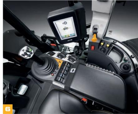
**6** Seat-mounted console houses the most frequently used control switches and dials with a generously padded armrest built in.
