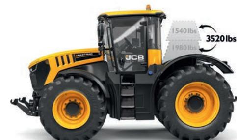
5 We all know that front axle suspension improves traction by eliminating power hop – well it's also true for rear axle suspension. That's one reason for the exceptional tractive effort generated by the Fastrac's tires.
