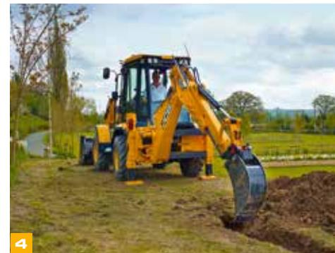
**5** Under 2 metre machine width gives it the ability to work in confined areas which are inaccessible to larger machines (attachment dependent).
