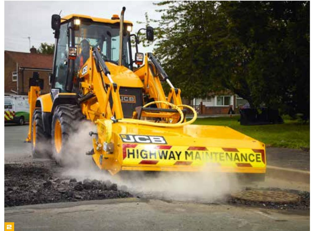
**3** A compact size allows it to work in confined areas that are inaccessible for standard size backhoes.
