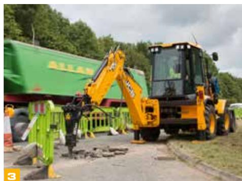
**4** Under 6 metre turning circle gives it the manoeuvrability to work in confined spaces.
