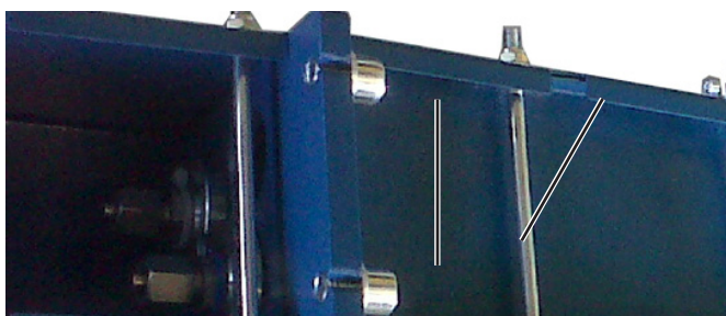
7 Tensioning plate 8 Fastening screws
