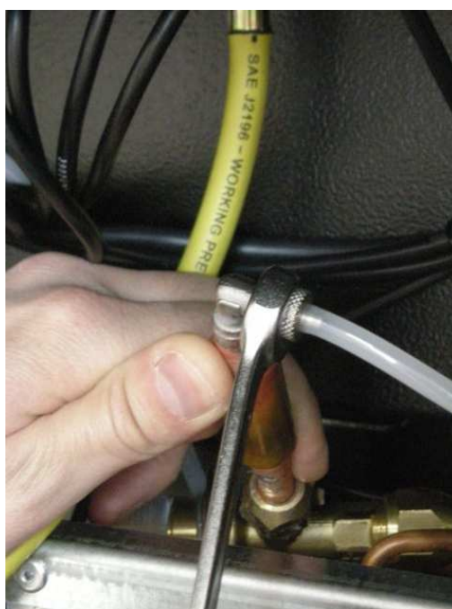
Image 7.16 – Removal of the small tube that leads the refrigerant from the HP/LP hoses to the mechanic filter
