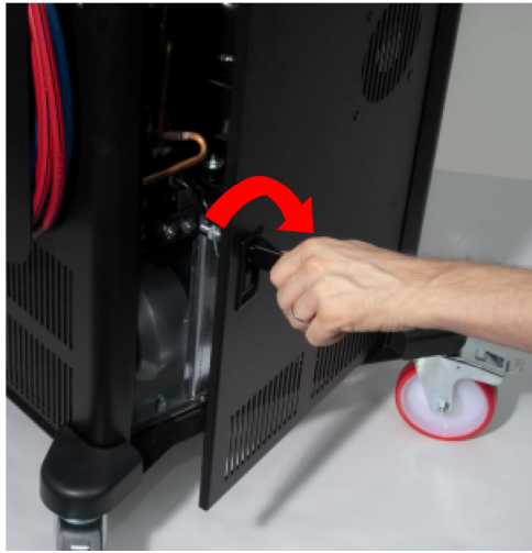
Image 5.7 – Opening of the service door located on the back of the Konfort unit
