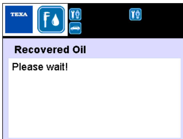
Image 4.73 - Waiting message during calibration of the drained oil load cell
