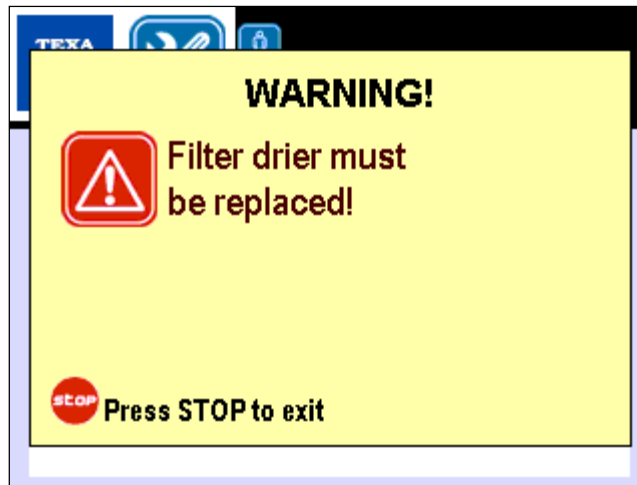
Image 5.2 – The main filter is completely exhausted. The unit cannot proceed with further recovery phases
