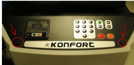
Image 4.19 – Screws removal from the top panel of the equipment
