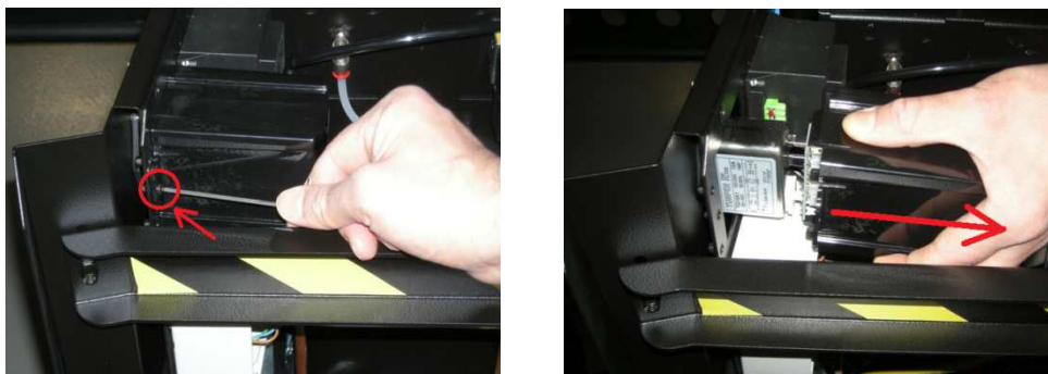
Image 7.1 – Removal of the cap of the network filter on Konfort 720R, 760R, 760R Bus and 780R BiGas
