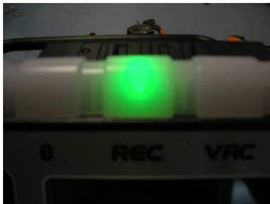
Image 6.6 – Flashing green REC led during the firmware update of the unit
