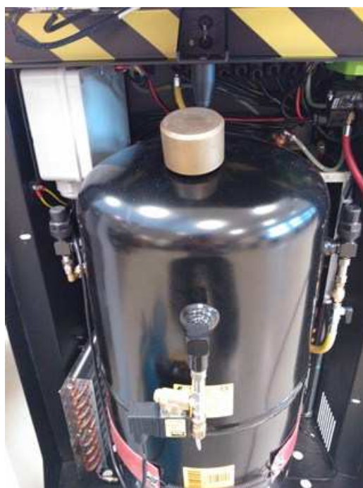
Image 4.51 – Positioning of a sample weight over the tank
