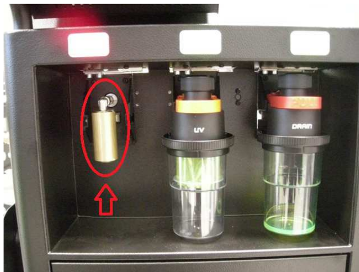
Image 4.80 – Connection of the 400-grams sample weight to the plug of the oil injection
