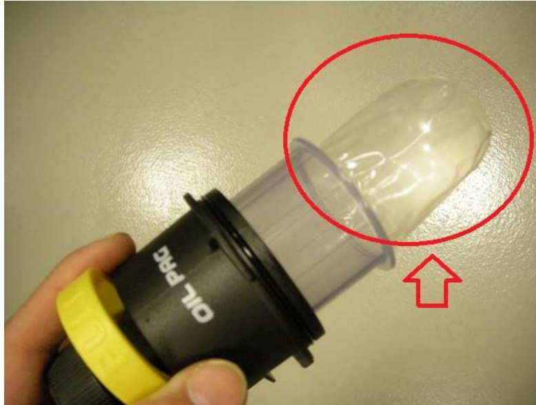
Image 7.27 – Check of the integrity of the inner membrane of the oil and UV injection bottles
