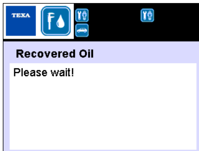
Image 4.71 – Waiting message during calibration of the drained oil load cell
