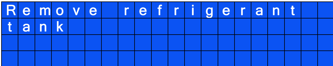
Image 4.24 – Request for removal of the refrigerant tank during the calibration of the load cell of a Konfort 705R, 710R or 720R
