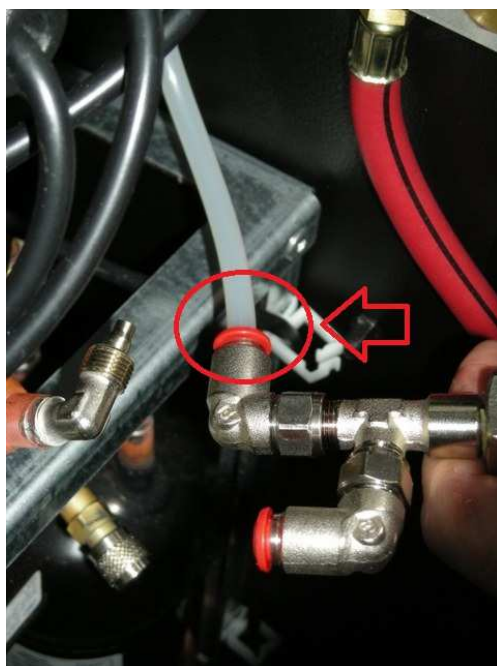
Image 7.18 - Connection of the silicone tube coming from the HP/LP hoses to the inlet of a vacuum gauge
