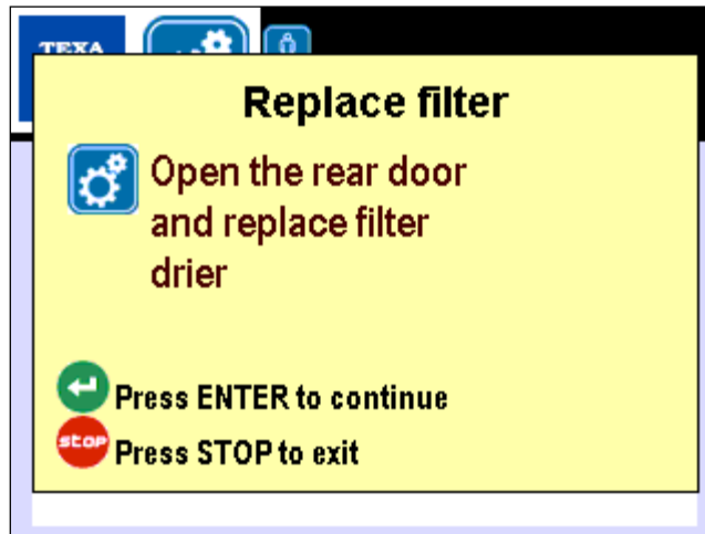
Image 5.5 – Request to open the back compartment in order to replace the main filter
