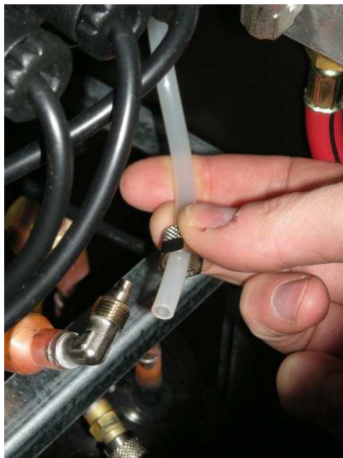
Image 7.17 - Small silicone tube coming from the HP/LP hoses disconnected from the mechanic filter
