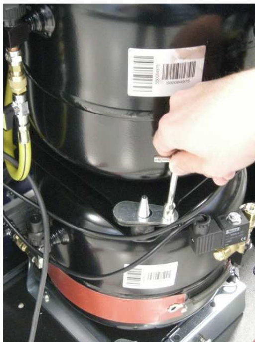
Image 4.65 – Removal of the blocking bracket from the upper tank of the Konfort 780R BiGas
