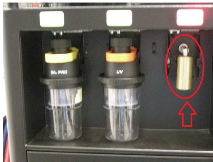
Image 4.75 – Connection of the 400-grams sample weight to the plug of the drained oil
