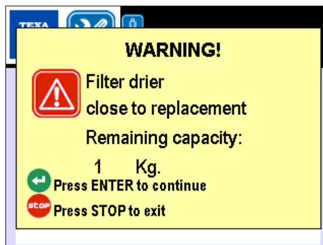
Image 5.1 – Warning message about the imminent exhaustion of the main filter
