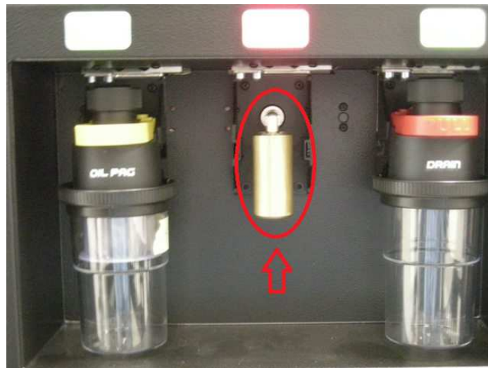
Image 4.79 – Connection of the 400-grams sample weight to the plug of the UV injection
