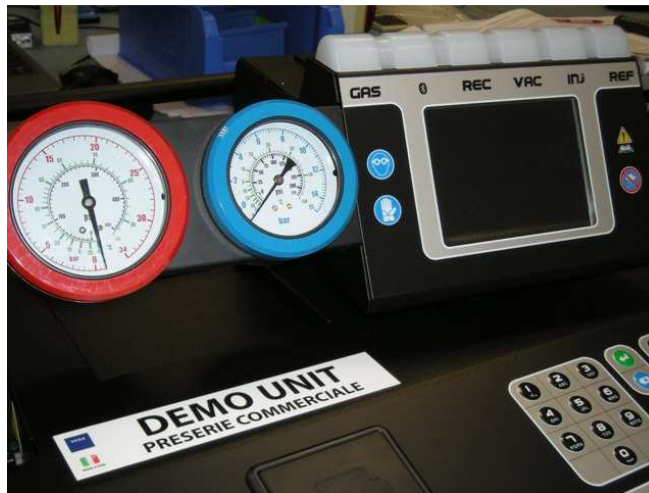
Image 7.12 – Black display accompanied by a “beep” while starting up a Konfort 760R, 760R Bus or 780R BiGas
