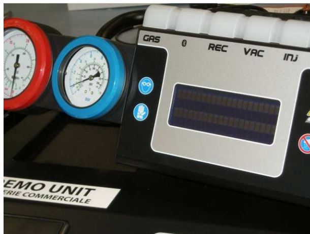
Image 7.10 - Backlight off accompanied by a “beep” while starting up a Konfort 720R
