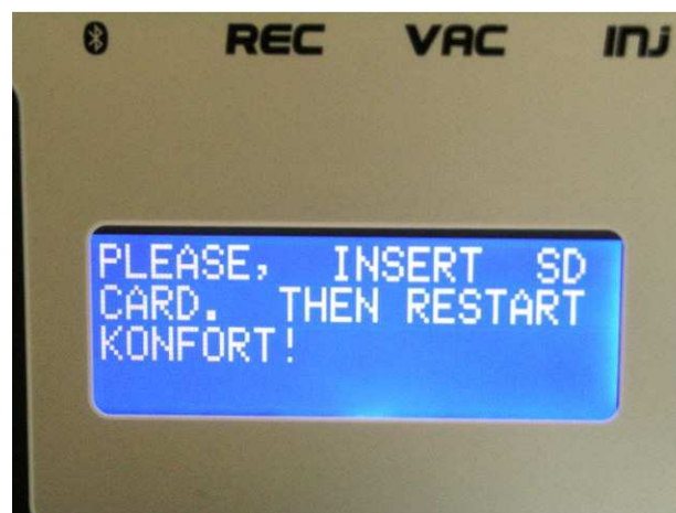
Image 7.8 - Request for SD insertion and no “beep” while starting up a Konfort 705R, 710R or 720R unit
