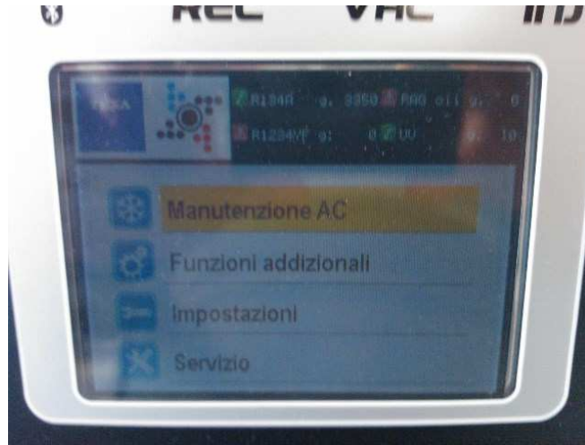
Image 7.15 – Display not enough bright (low backlight) on Konfort 760R, 760R Bus or 780R BiGas
