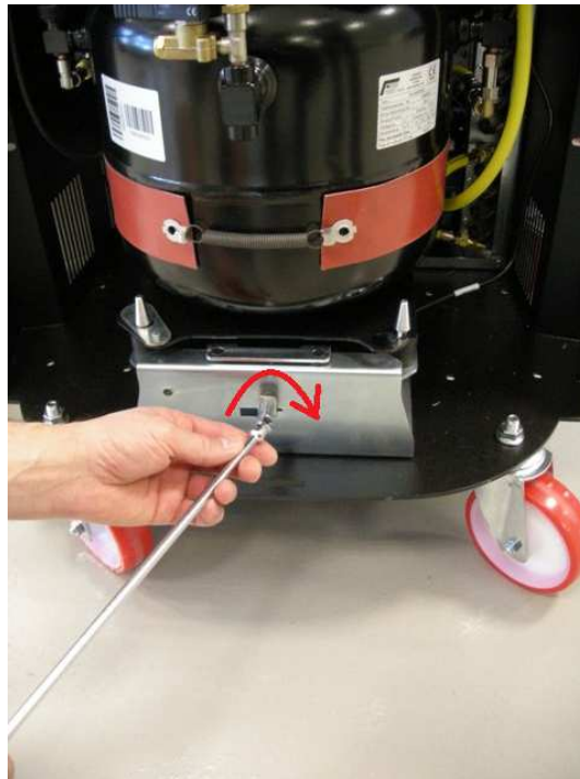
Image 4.56 – Scale lock on a Konfort 780R BiGas
