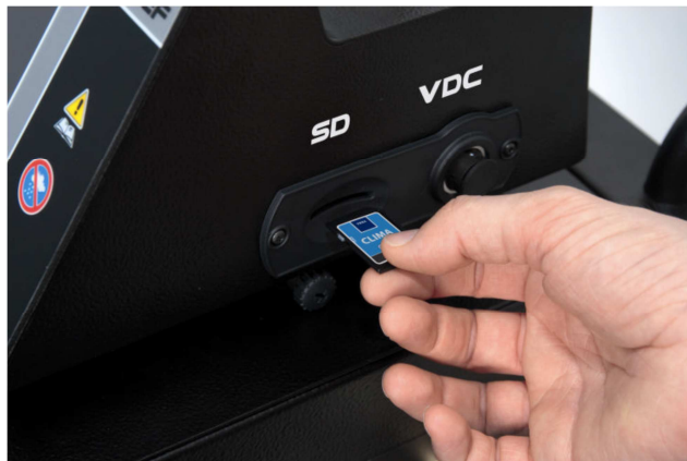
Image 6.10 – SD card removal from the Konfort 700R
