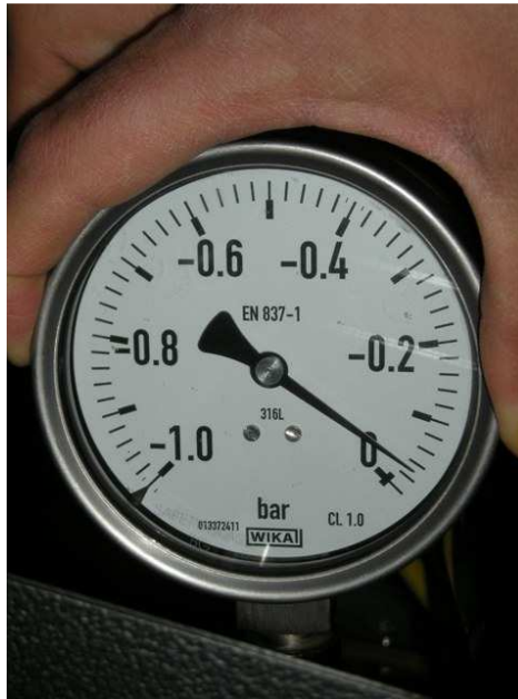
Image 7.21 – Very low depression level showing a possible suction problem
