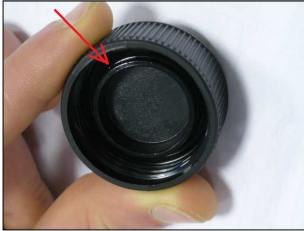
Image 7.28 – Check of the o-ring inside the upper cap of the injection oil bottle
