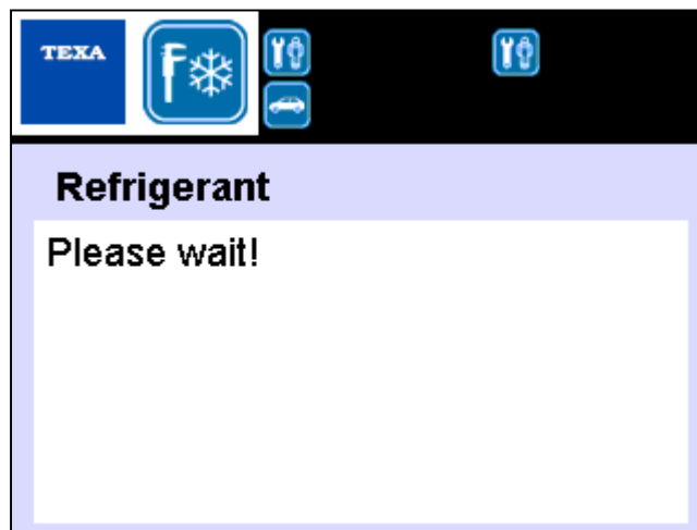
Image 4.69 – Waiting message during calibration of the main load cell
