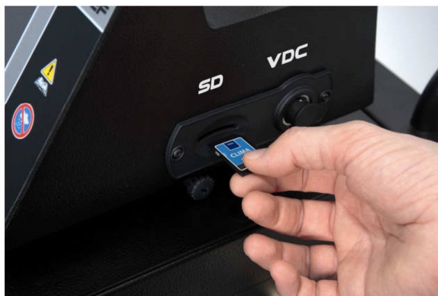
Image 6.3 – SD card removal from the Konfort 700R
