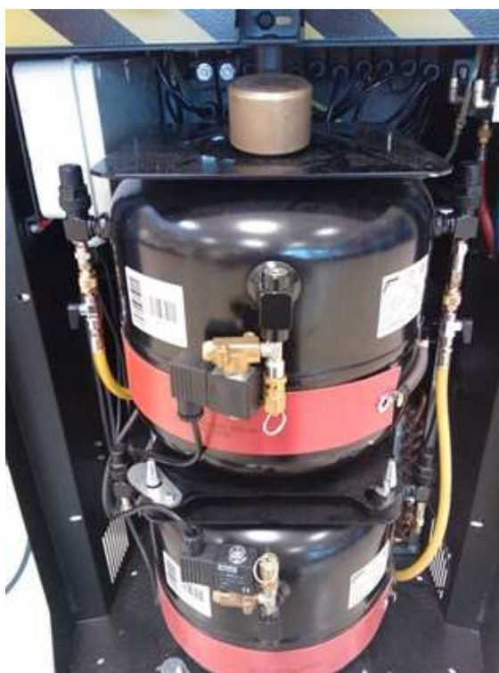
Image 4.61 – Positioning of a sample weight over the upper tank of 780R BiGas
