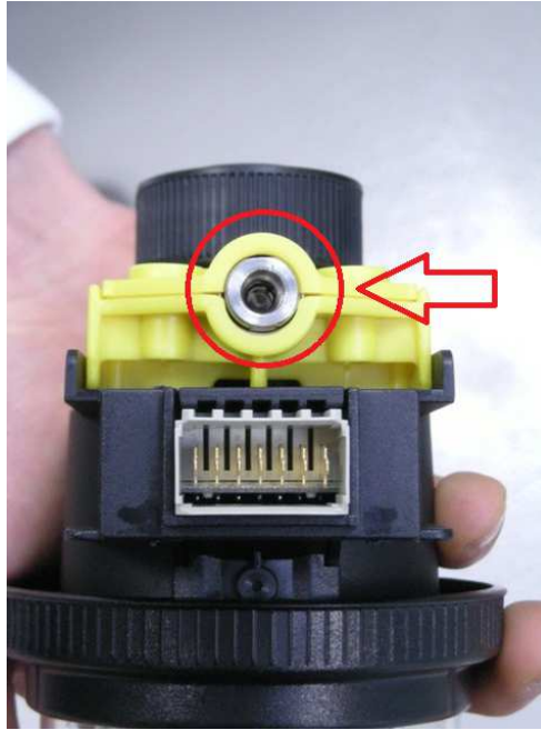
Image 7.30 – Check that the quick connector on the oil injection bottle will not be obstructed
