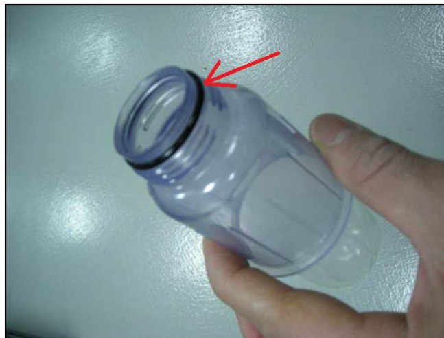
Image 7.29 – Check of the o-ring located on the upper part of the inner container with membrane
