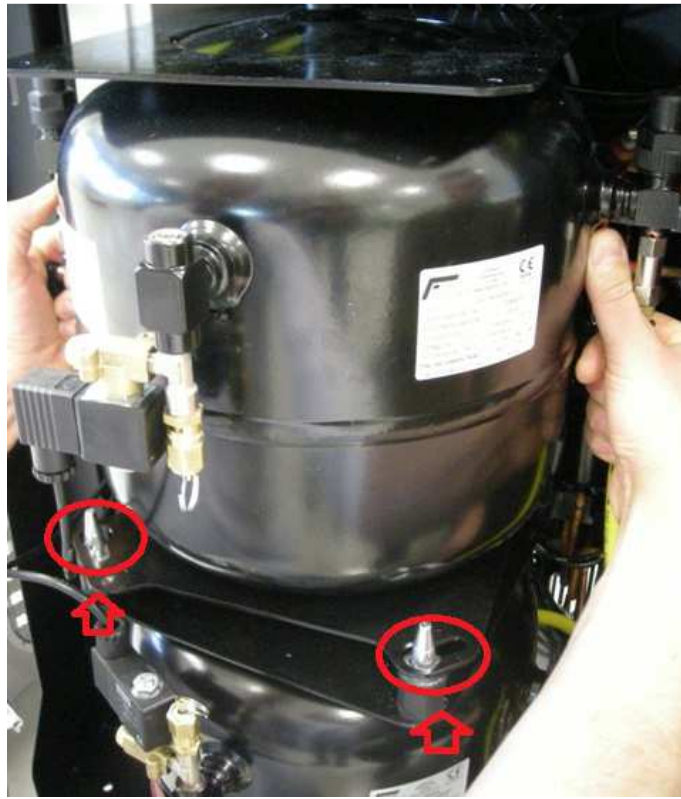
Image 4.66 – Raising of the upper tank from the lower one of the Konfort 780R BiGas
