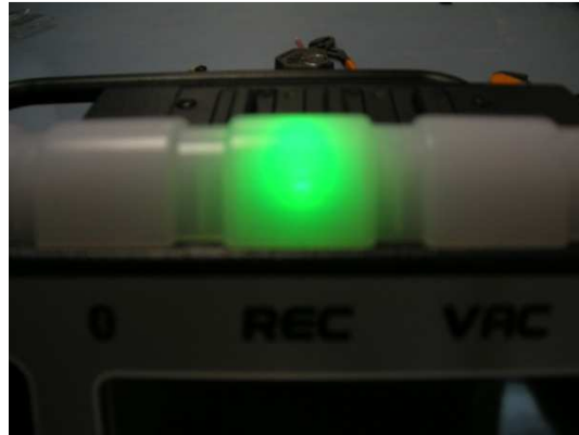
Image 6.15 – Flashing green REC led during the firmware update of the unit
