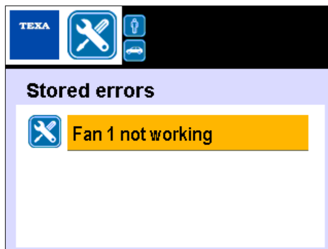
Image 4.89 – Example of the Stored errors function on Konfort 700R units
