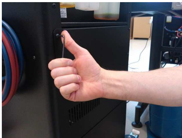
Image 5.6 – Opening the back compartment on Konfort 710R
