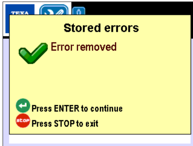
Image 4.92 – Confirmation of the stored error deletion. Press the ENTER button for quitting the page
