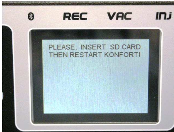
Image 7.9 – Request for SD insertion and no “beep” while starting up a Konfort 760R, 760R Bus or 780R BiGas unit
