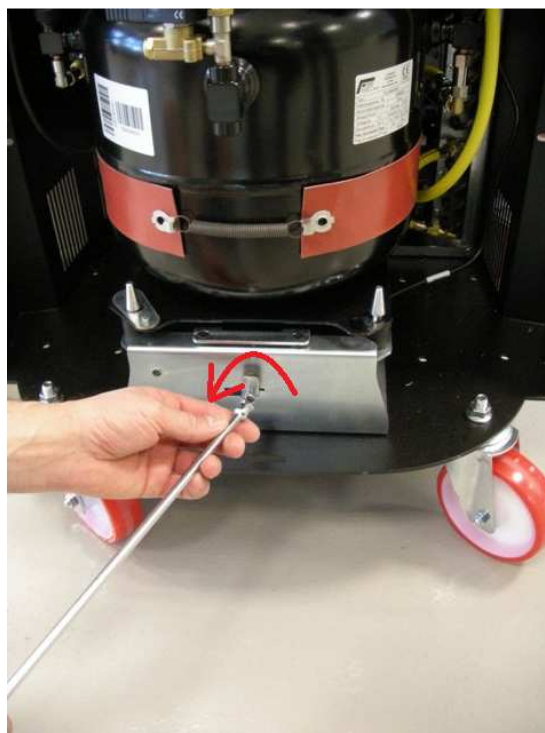
Image 4.59 – Scale unlock on a Konfort 780R BiGas
