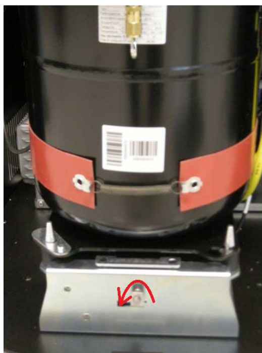
Image 4.49 - Refrigerant scale unlock
