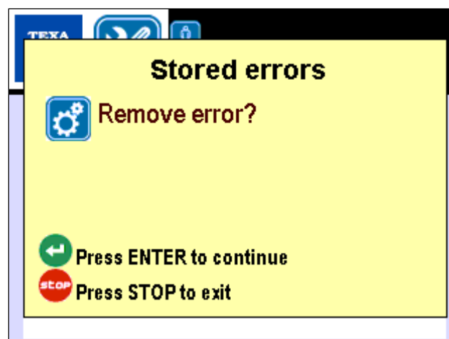
Image 4.91 – Request for stored error deletion by pressing the ENTER button
