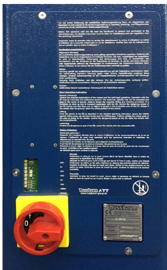
Figure 4: Operating unit with reversing switch (2.30 SL to 2.40 SL)
