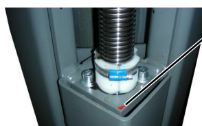
Figure 18: The lift nut pin is provided with a sealing wax
