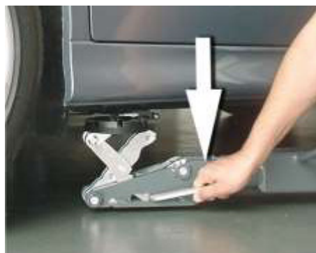
Figure 2: If required, place the carrier plate by pushing the lever at the fixture points
