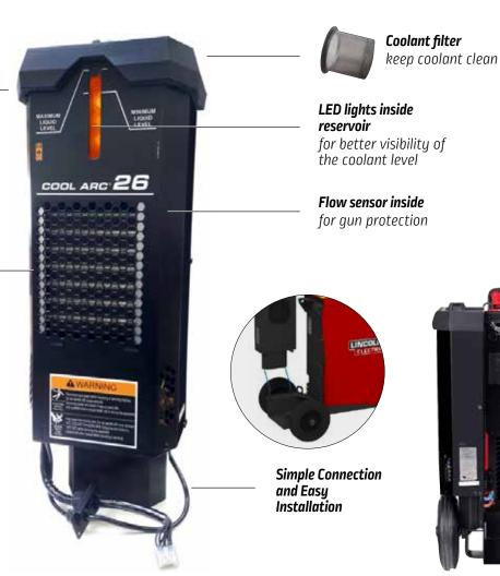
Weight (kg) Dimensions Protection **Cooling power** Reservoir Product Input (V) Item Number @1L/min (kW) WxLxD(mm) capacity (L) Class 230/400V COOLARC<sup>®</sup> 26 IP23 K14182-1 ±15% 0.84 4 18 260 x 150 x 680 50/60 Hz
