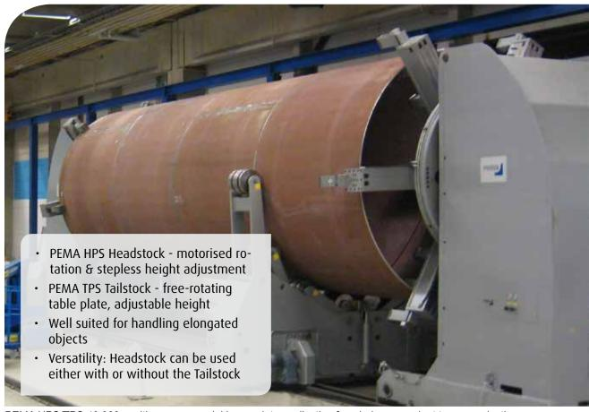
PEMA HPS/TPS 40 000 positioners, a special heavy-duty application for wind energy plant tower production
