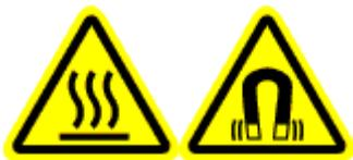
**Do not wear clothing that is made with metallic pocket rivets, waist band buttons, pocket buttons, and zippers when operating the Mini-Ductor® Venom™.** The Mini-Ductor® Venom™ can heat such metallic items very quickly and cause serious burns or even ignite clothing.
