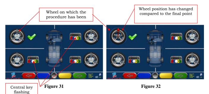
On Figure 31 the front left wheel is shown with a tick on the side, to indicate that the procedure has been carried out on that wheel. Procedure can anyway be repeated by pressing again the central key of the concerned detector. When the Run-Out procedure has been completed on all wheels, programme will automatically go to the next phase.
