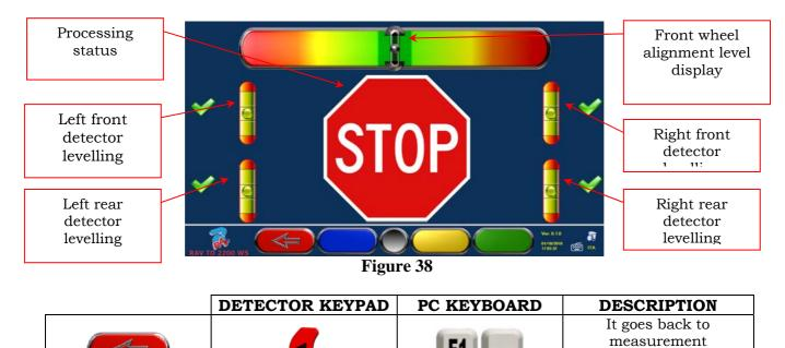
Turn steering wheel from left to right, or vice-versa, until wheels are aligned, namely until display level is not perfectly centred.
