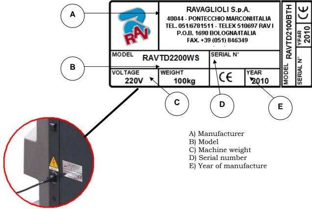
WARNING: It is strictly forbidden to tamper with, notch, somehow alter or even remove machine identification plate; do not cover it with temporary panels, etc... as it shall always be clearly visible.
