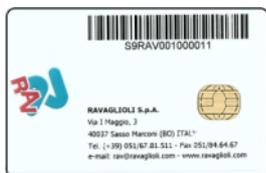
**WARNING:** Before switching the machine on, make sure that the **SMART CARD** for programme enabling and the database are in the special reader on PC front side.
