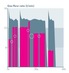
Comparison of the gas consumption with and without the  $\ensuremath{\mathsf{EWR}}$  system
